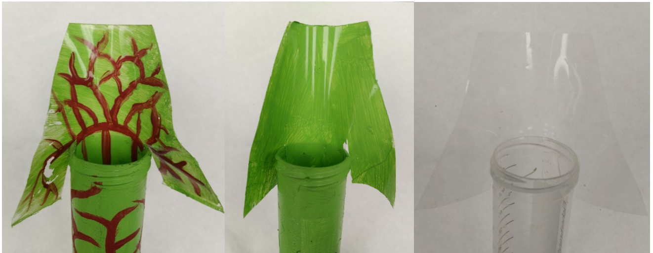
Figure 2. Example ‘pseudopitchers’ made of 50 mL Falcon tube and a sheet protector ‘hood’. From left to right: pitcher with red veins, pitcher with only green (“sans veins”) and colorless control.
